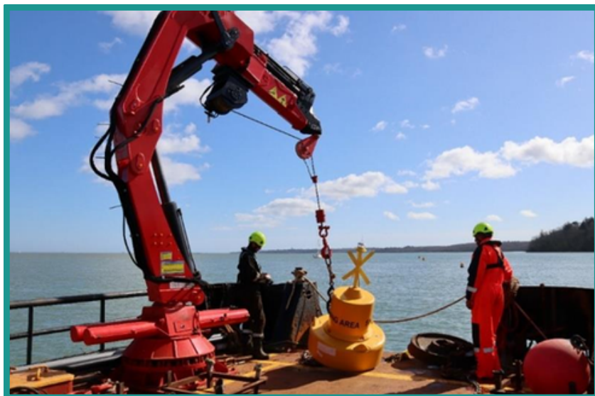
Vessel installing marker buoy with a train wheel sinker in Osborne Bay. Credit: Andrew Hunt, VSEL
